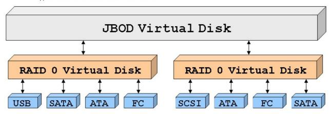
VxWorks RAID virtual disks can be created using any combination of Block Devices such as USB, ATA, SATA, SCSI and Fiber Channel.
